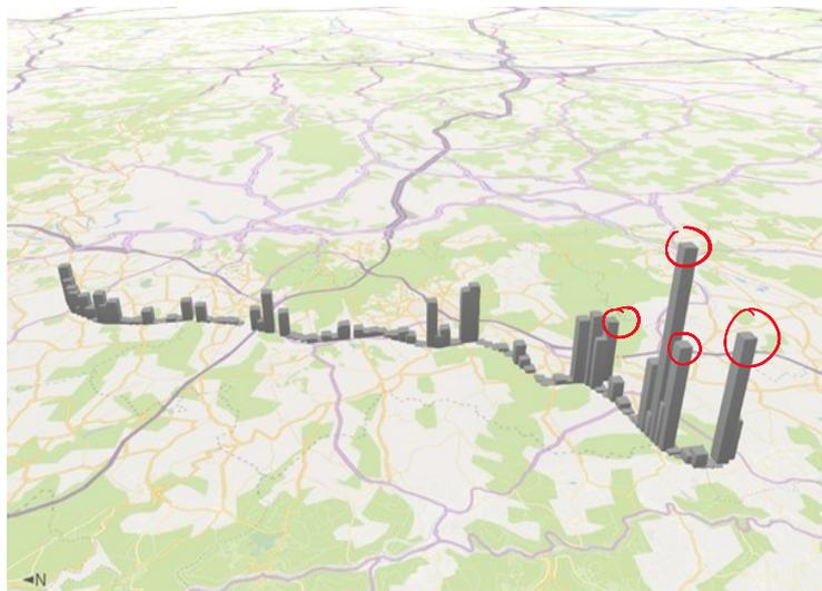
*Figure 1 – A procedure to locate the hotspots on a line route, i.e. the places where the conductor temperature tends to be higher than the rest of the line, was created and tested on a sample overhead line in Germany. After locating the hotspots, the installation places for the weather stations can be determined based on a given budget.*
